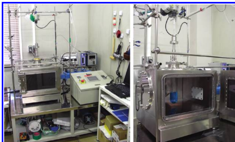
Figure 9. Pictures of the SMW-101 MW reactor showing the entire instrument (left) and the reaction cavity (right).
